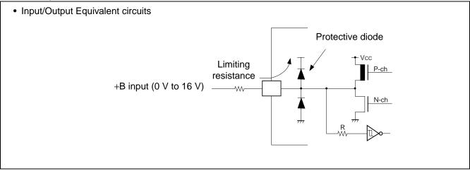
\*8: P24 to P27, P30 to P37, P40 to P42, P70 to P74, P76, P77 pins can be used as 5 V I/F pin on applied 5 V to Vcc5 pin.
