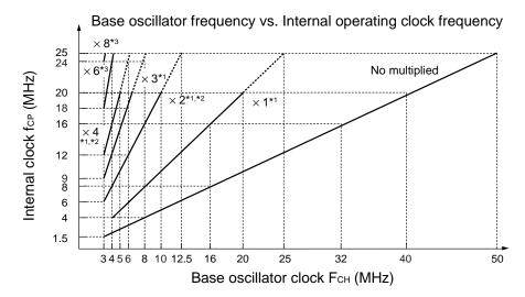
\*1 : In setting as 1, 2, 3 and 4 multiplied PLL, when the internal clock is used at 20 MHz < fcp ≤ 25 MHz, set the PLLOS register to "DIV2 bit = 1" and "PLL2 bit = 1".
