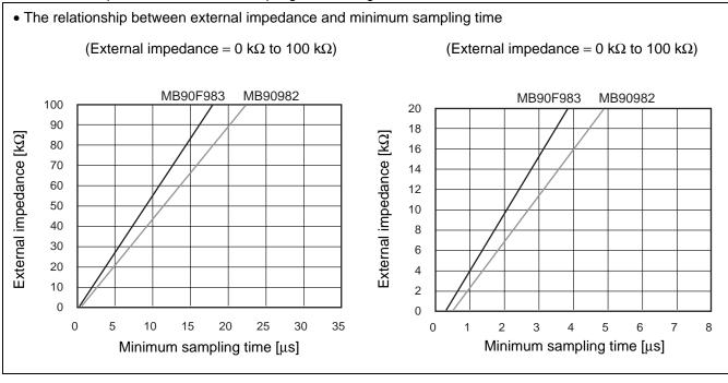
• If the sampling time cannot be sufficient, connect a capacitor of about 0.1  $\mu F$  to the analog input pin.
