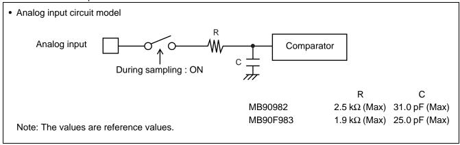
• To satisfy the A/D conversion precision standard, consider the relationship between the external impedance and minimum sampling time and either adjust the resistor value and operating frequency or decrease the external impedance so that the sampling time is longer than the minimum value.
